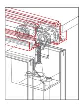
Designed to accommodate suspended ceilings. Installation can include track support and sound baffles within ceiling voids according to specification.
